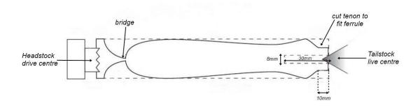
5] Finish by pushing the ferrule over the tenon and gluing the handle shaft of the kit into the handle. The ferrule does not need to be glued in place, the main scoop will prevent it from slipping off and the ferrule will prevent the wood from splitting from internal pressure from the shaft.
